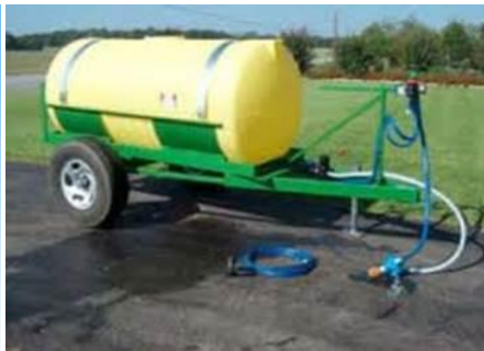
Trailer Sprayer (with Snyder Super poly Tank)
