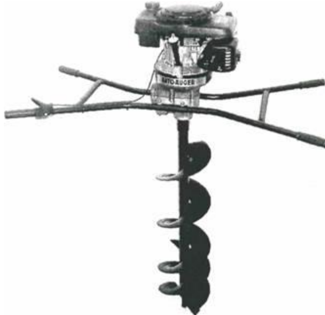
Engine operated post hole digger - manual handling
