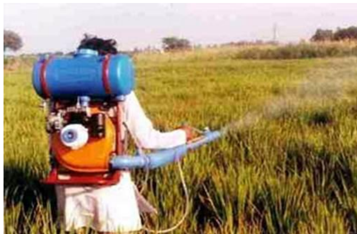
Motorized Knapsack sprayer spraying chemicals to wheat crop.
