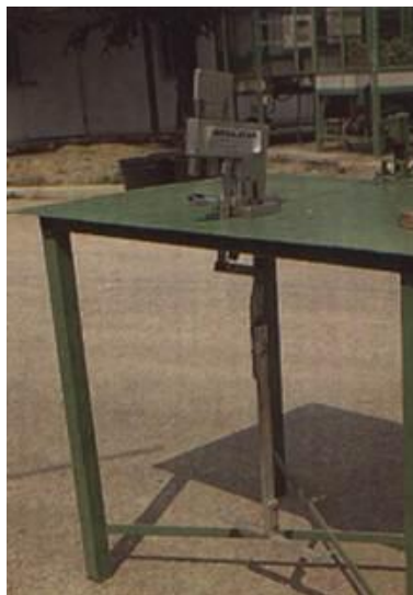
Saw type electrically powered grafting machine
