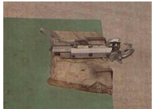
Foot operated bench grafting tool- omega cut
