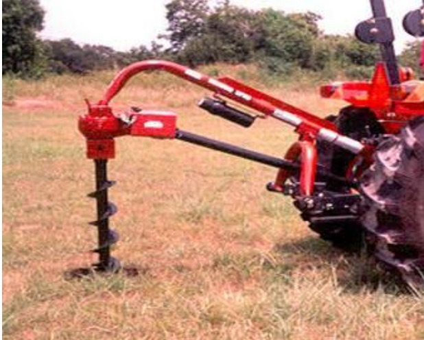
Tractor operated Post hole digger- gear drive
