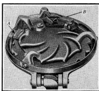
Fig. 11.4. Left: Hopper bottom for typical horizontal-plate corn planter. Note the spring-loaded (yielding) cutoff A, and the spring-loaded knockout pawl B. Right: Three types of edge-cell plates used interchangeably in this hopper bottom. (International Harvester Co.)
