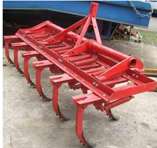
Tractor drawn cultivator- spring loaded tines
