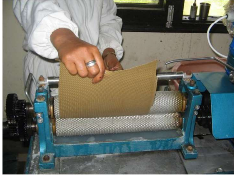
Figure 6.5 Comb Foundation Mill
