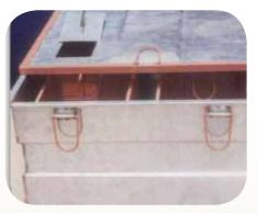
three inner containers to hold rhizomes. Washed rhizomes are loaded in the inner cylinder and required quantity of water is added in the outer cylinder. Rhizomes are boiled by the steam liberated from the boiling water. Sodium bicarbonate is added in the boiling water to add colour. The inside containers which hold turmeric can easily be taken out without wasting boiling water, which can be reused and thereby fuel requirement can be considerably reduced.
