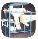
power operated green pea pod sheller to meet the requirement of the pea growers. The sheller consisted of feeding hopper, roller, concave, frame and a 0.25 hp electric motor. The roller is fixed on a central shaft supported on two bearings. The roller rotates in the concave. The roller and concave assembly are mounted on a frame. The concave consists of galvanized iron sheet punched with holes of 16mm dia. at a centre to centre distance of 26 mm.
