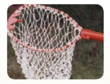
cutting the petiole of the fruit. Nylon net is fixed to the metal ring to hold the plucked fruits. The unit needs to be fixed to a long pole of suitable length to reach the fruits on the tree.
