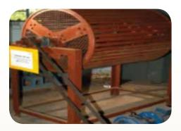
the individual cups in hand. To overcome this problem, a power operated coconut de-shelling machine was designed and developed. The capacity of the machine is 400 half cups per batch. The optimum average moisture content for maximum de-shelling efficiency (92.16 %) is 35 % d.b. The optimum speed of the de-shelling machine is 10 RPM and the time taken for de-shelling is 4 minutes per batch.
