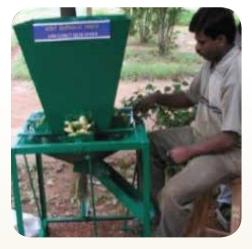
sembly consists of two sharp edged blades, one being stationary and the other movable, operated by a pedal through a linkage mechanism. The unit has a hopper to hold 20kg raw nuts and the raw nut freely flows to the de-husking tray by gravity. The outer shell of freshly harvested nut is pierced by pressing the nut against the sharp edge of the blade and the leg pedal is operated to split the husk. About 2-3 strokes are required to completely de-husk a nut.
