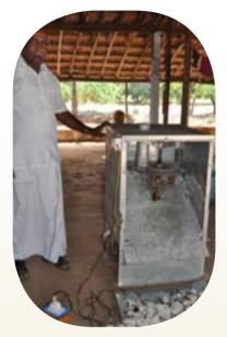
cut pieces are placed in the tray of the machine for easy hand picking. Later, the chips shall be uniformly dried and hence, degradation of starch is reduced this is the main advantage in this value addition. The size of the chips ranges from 2mm to 25 mm thickness.
