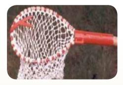
one end for cutting the petiole of the fruit. Nylon net is fixed to the metal ring to hold the plucked fruits. The unit needs to be fixed to a long pole of suitable length to reach the fruits on the tree.
