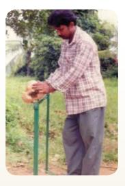
a portion of the husk. The operation is repeated 3-4 times until complete de-husking is done.
