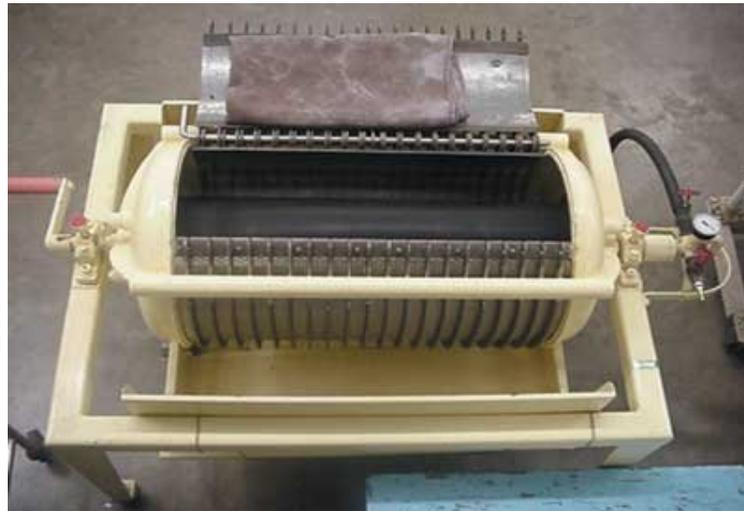
**Figure 1.11: Bladder press, 100L capacity.**
