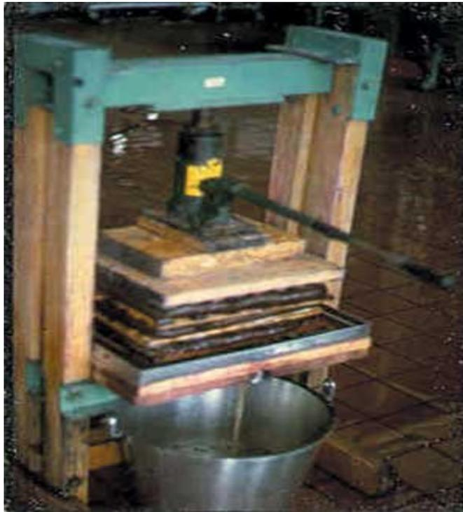
Figure 1.10: Simple hydraulic rack and cloth press.
