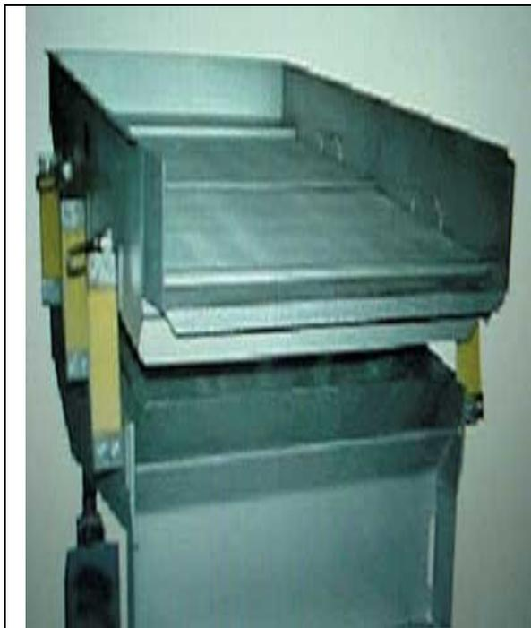
**Figure 1.13b: Shaker separating screen used in conjunction with a continuous centrifuge.**
