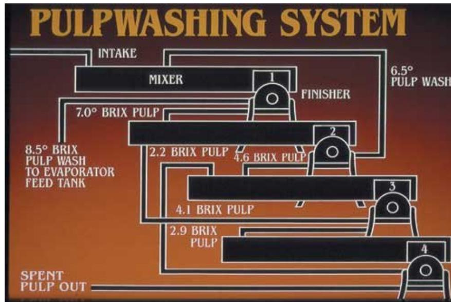
Figure 1.7: Pulp wash extraction schematic.
