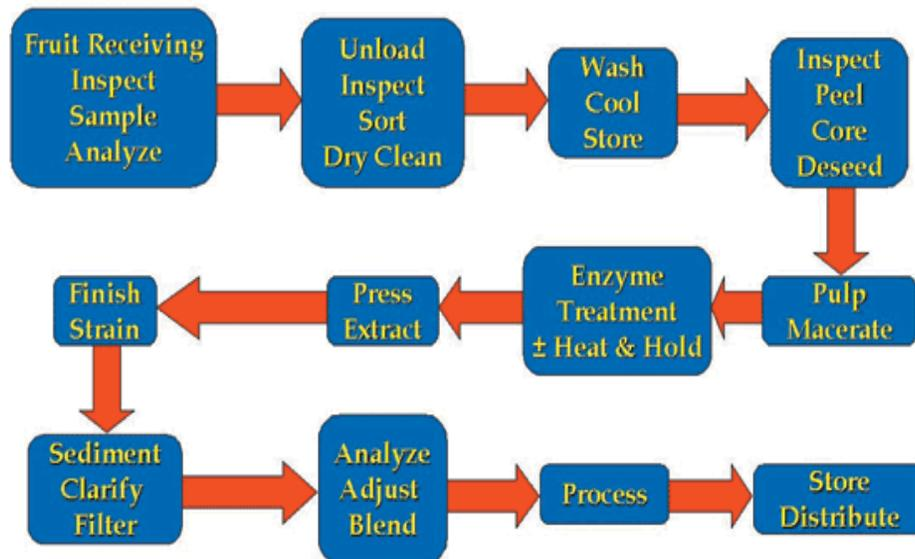
Figure 1.1: Generalized juice flow scheme.
