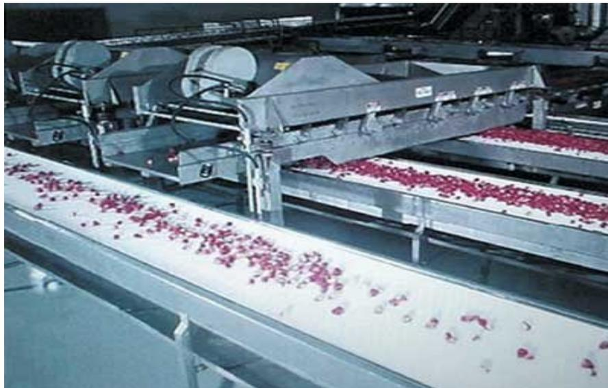
**Figure 1.3: Automatic inspection/grading system.**
